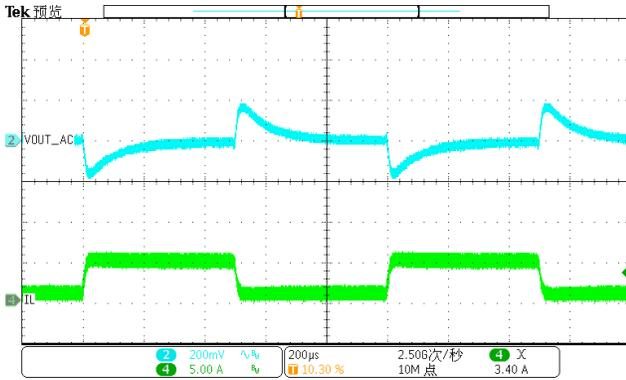
Figure 19. Load Transient (0.5A-4.5A, 1.6A/us)
