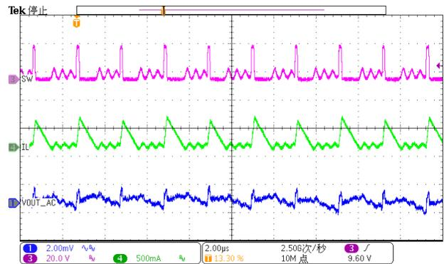
Figure 22. Output Ripple (Iload=100mA)
