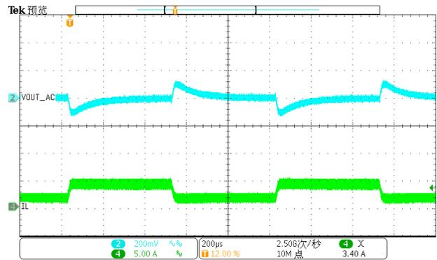
Figure 20. Load Transient (1.25A-3.75A, 1.6A/us)
