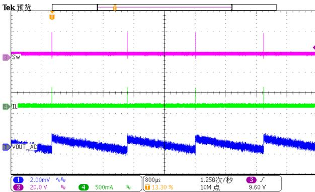
Figure 21. Output Ripple (Iload=0A)
