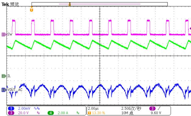
Figure 23. Output Ripple (Iload=5A)
