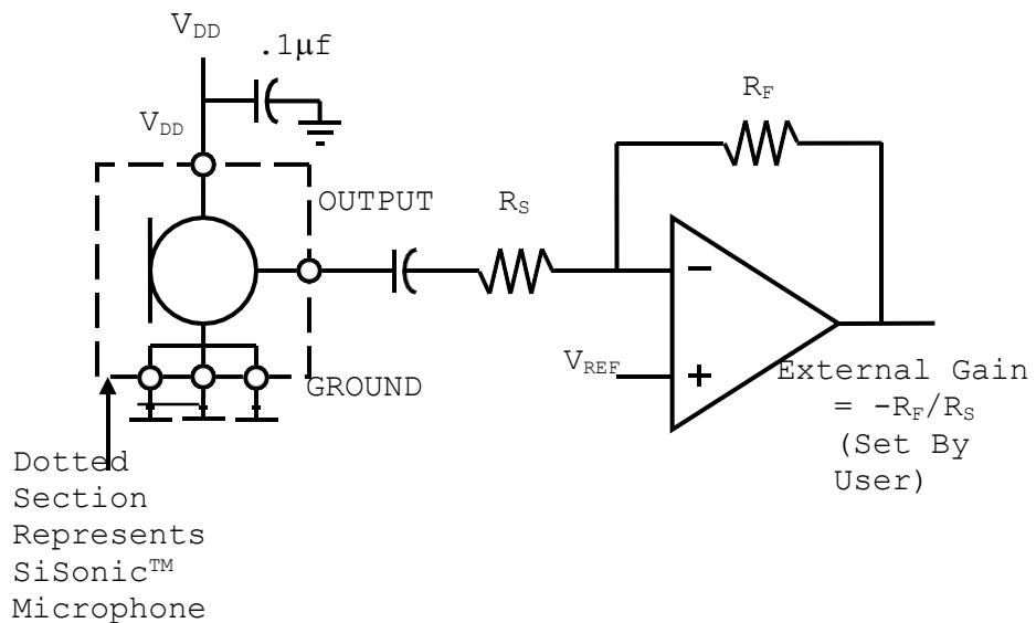
Notes: All Ground pins must be connected to ground.
