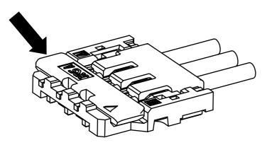
② Lift up to the upper difrection and friction lock
