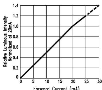
Fig.4 Relative Luminous Intensity
