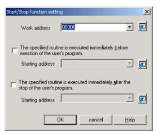
Figure 5.123 Start/Stop function setting dialog box
