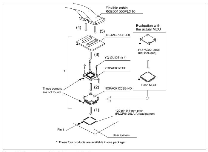
Figure 2.11 Connection to a 120-pin 0.4-mm pitch pad pattern
