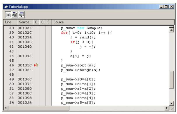
Figure 3.27 Editor window (setting a hardware breakpoint)
