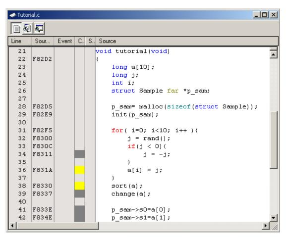
Figure 5.87 Example of code coverage results
