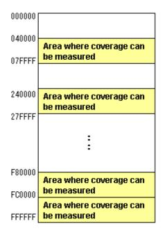
Figure 5.74 Schematic view of coverage memory allocation
