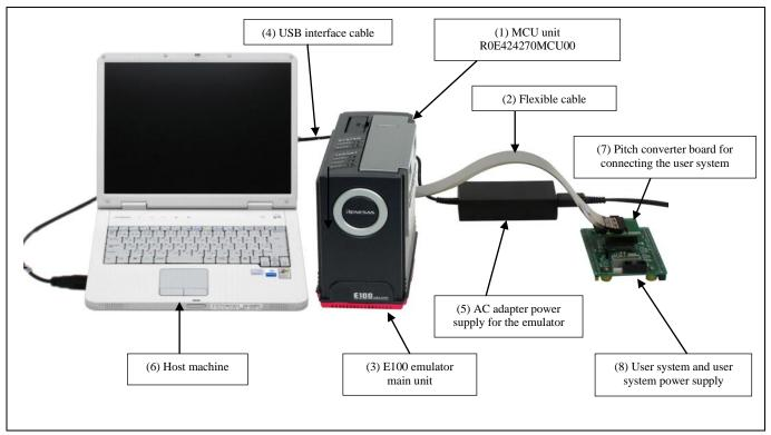
Figure 1.1 System configuration
