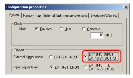
Figure 5.124 Configuration properties dialog box (System page)
