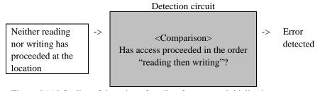
Figure 5.115 Outline of detection of reading from a non-initialized area
