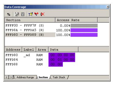
Figure 5.93 Data Coverage window (section name specification)
