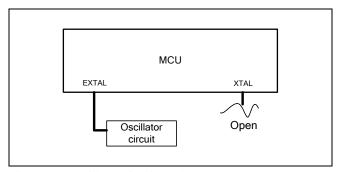
Figure 2.8 Oscillator circuit on the user system
