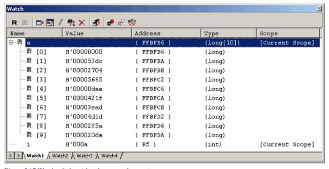
Figure 3.17 Watch window (showing array elements)
