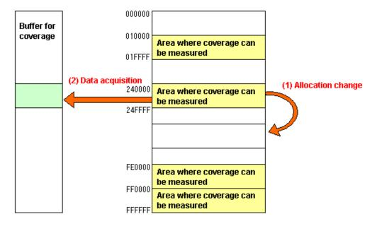
Figure 5.91 Schematic view of a change in data coverage memory allocation
