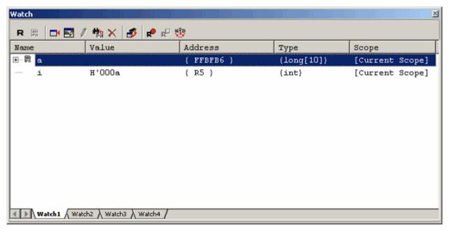
Figure 3.16 Watch window (showing a variable)
