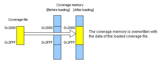
Figure 5.84 Schematic view of the overwrite mode
