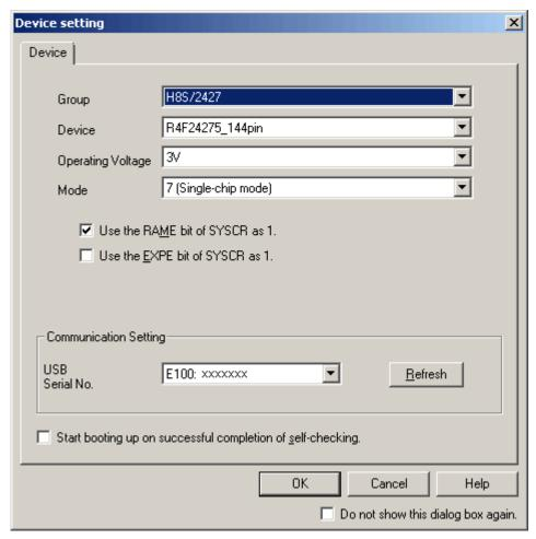
Figure 5.1 Device setting dialog box (Device page)
