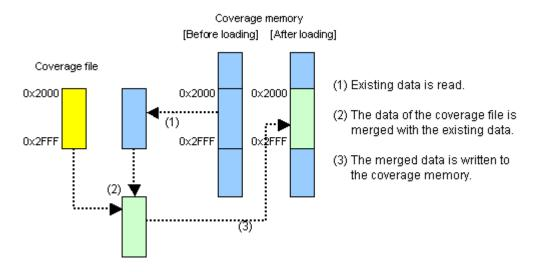
Figure 5.85 Schematic of the merge mode
