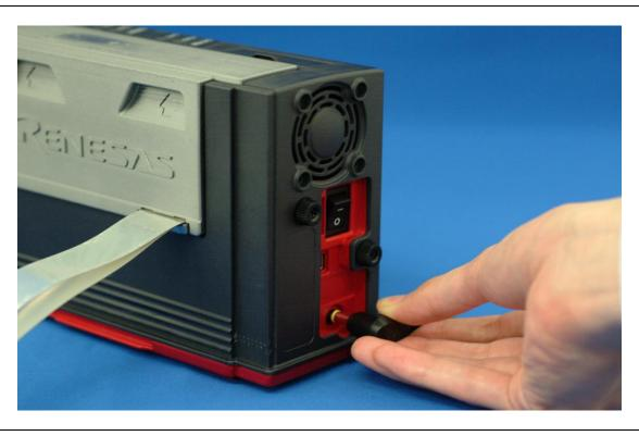
Figure 2.5 Connecting the emulator power supply
