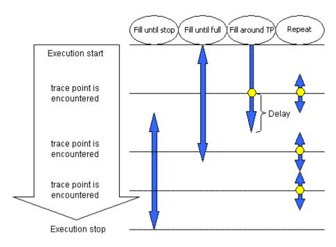
Figure 5.49 Differences between the trace modes
