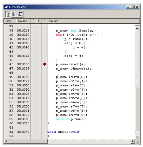
Figure 3.4 Editor window (setting a software breakpoint)
