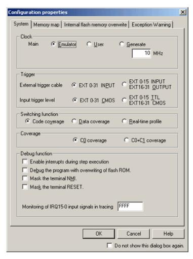
Figure 5.2 Configuration properties dialog box (System page)
