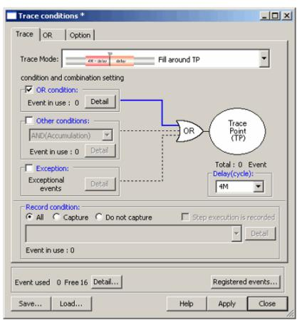
Figure 3.34 Trace conditions dialog box (Fill around TP)
