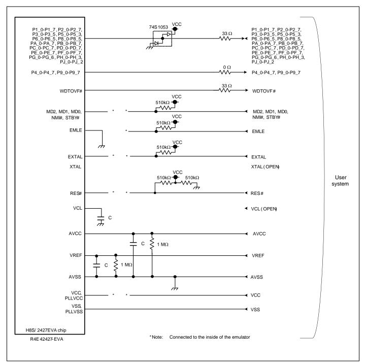
Figure 7.1 Connection diagram for R0E424270MCU00
