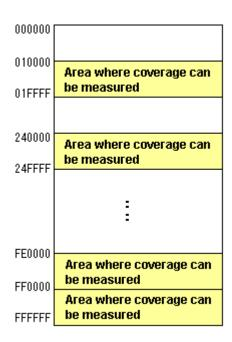
Figure 5.90 Schematic view of data coverage memory allocation
