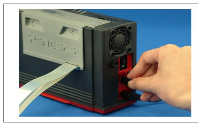
Figure 2.4 Connecting the host machine
