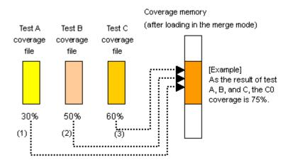
Figure 5.86 Schematic view of a merge-mode application
