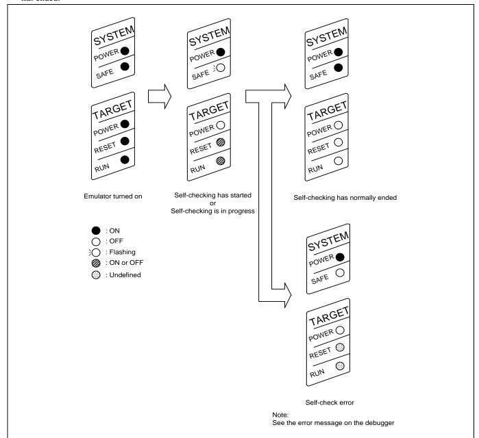
Figure 2.6 LEDs during self-checking
