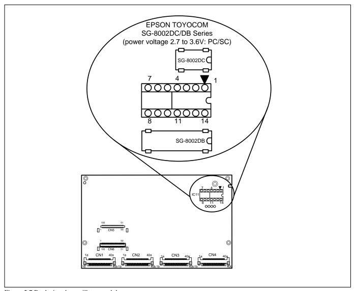
Figure 2.7 Replacing the oscillator module
