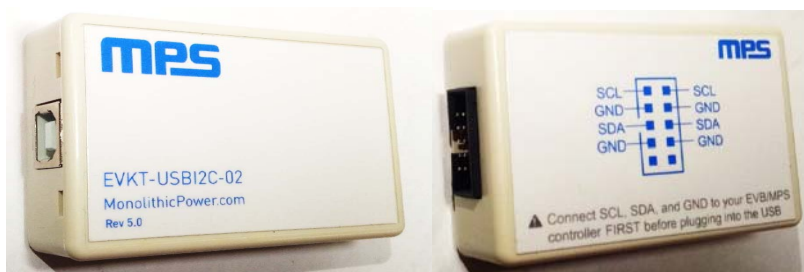
Figure 1: USB to I 2 C Communication Interface
