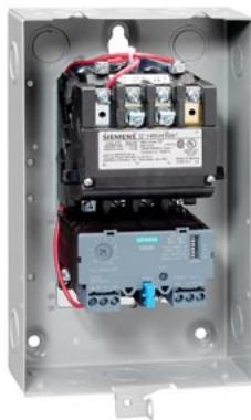
Non-reversing motor starter, Size 1, Three phase full voltage, Solid-state overload relay, OLR amp range 10-40A, 208VAC 60Hz coil, Non-combination type, Enclosure type 1, Indoor general purpose use, Extra-wide enclosure
