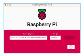
Now click on storage to open the available USB devices which in my case only shows the CM4Stack. Click on it to select it and click "Write to begin installing the new OS version.
