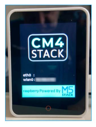
In the above image you can see that the CM4Stack is connected via wlan0 but I have blurred out the IP address for privacy.
