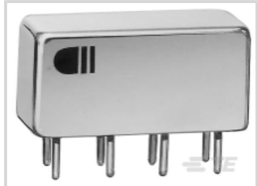
1/5-Size Relay Contact Arrangement: **2 Form C, DPDT, 2 C/O**1/5-Size Relay Input Voltage: **26.5 VDC**Coil Suppression Diode: **With**1/5-Size Relay Contact Current Rating: **2 A**1/5-Size Relay Coil Voltage Rating: **26.5 VDC**
