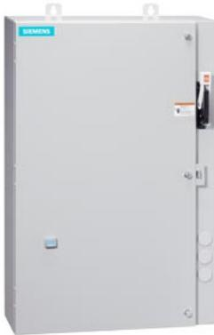
Reversing motor starter, Size 1, Three phase full voltage, Solid-state overload relay, OLR amp range 0.75-3.4A, 110V 50Hz / 120V 60Hz coil, Combination type, 30A disconnect switch, Enclosure NEMA type 4/12, Water/dust tight for outdoors
