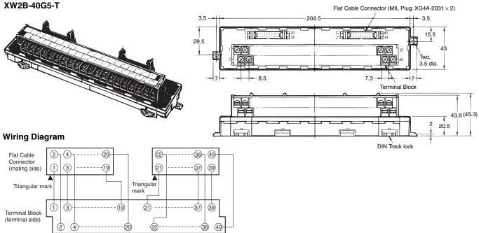
Note: All pins on the Flat Cable Connector correspond 1-to-1 to the terminal of the same number on the terminal block as shown above.
