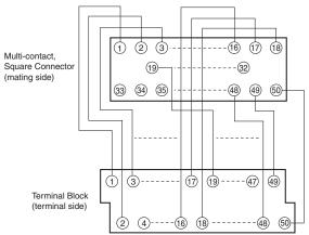
Note: All pins on the Multi-pole, Square Connector correspond 1-to-1 to the terminal of the same number on the terminal
