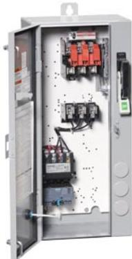
Non-reversing motor starter Size 1 Three phase full voltage Solid-state overload relay OLRelay amp range 10-40a 220-240/440-480VAC 60HZ coil Combination type 60Amp fusible disconnect 60Amp / 250V fuse clip Enclosure NEMA type 4/12 Water/dust tight weather proof Standard width enclosure
