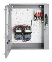
2-speed 3-phase motor starter Size 0 One winding consequent pole Constant or variable torque Solid-state overload relays Low SPD OLR range 0.25-1A High SPD OLR range 0.75-3.4A 110V 50HZ / 120V 60HZ coil Combination type 30Amp disconnect switch Enclosure NEMA type 1 Indoor general purpose use
