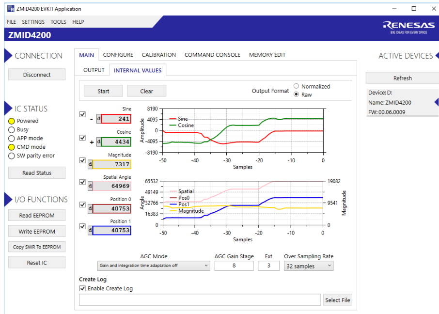
Figure 12. “INTERNAL VALUES” Tab – Analog Output Example
