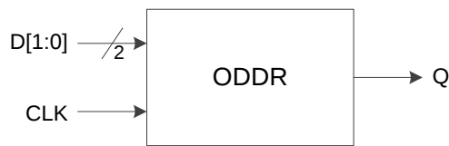
Figure 3-17 I/O Logic in DDR Output Mode
