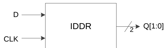
Figure 3-16 I/O Logic in DDR Input Mode
