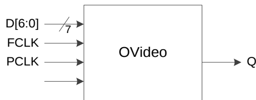
Figure 3-21 I/O Logic in OVideo Mode
