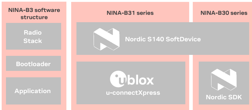
Figure 2: NINA-B3 software structure and available software options
