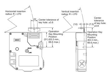
D4JL + D4JL-K3 (with Front-inserted Operation key)
