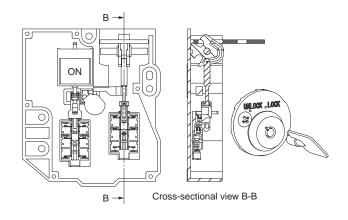
(3) Operation Key inserted, solenoid OFF, and trapped key inserted. Status: Door locked and trapped key cannot be removed.
