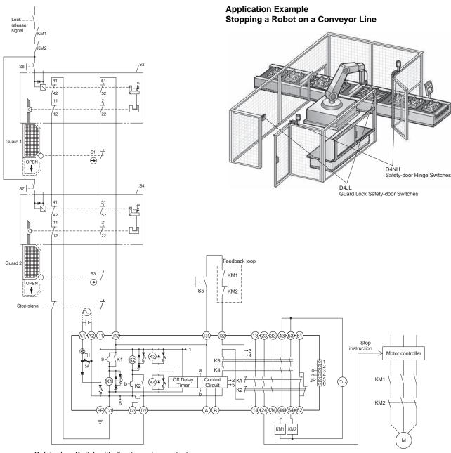
S1: Safety-door Switch with direct opening contact
