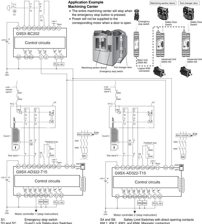
S3 and S7: Guard Lock Safety-door Switches S2, S5, and S9: Reset switches
