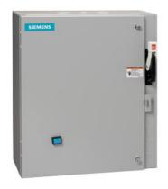
Non-reversing motor starter Size 3 Three phase full voltage Solid-state overload relay OLRelay amp range 25-100A 190-220/220-240V 50/60HZ coil Combination type 100A fusible disconnect 100A/600V fuse clip Enclosure NEMA type 1 Indoor general purpose use Standard width enclosure
