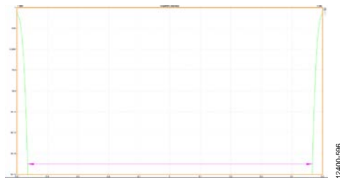
Figure 137. Bathtub, External 100Ω Terminations at 6 Gbps
