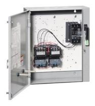
2-speed 3-phase motor starter, Size 1, Two separate windings, Constant or variable torque, Solid-state overload relays, Low Spd OLR range 0.75-3.4A, High Spd OLR range 3-12A, 110V 50Hz / 120V 60Hz coil, Combination type, 10A circuit breaker, Enclosure NEMA type 1, Indoor general purpose use
