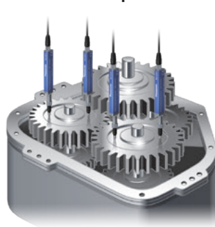
Transmission parts height measurement
