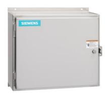
2-speed 3-phase motor starter, Size 0, One winding consequent pole, Constant or variable torque, Solid-state overload relays, Low Spd OLR range 0.75-3.4A, High Spd OLR range 0.75-3.4A, 110V 50Hz / 120V 60Hz coil, Enclosure NEMA type 12, Dust/drip proof for indoors
