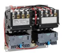
2-speed 3-phase motor starter Size 2 1/2 One winding consequent pole Constant or variable torque Solid-state overload relays Low SPD OLR range 25-100A High SPD OLR range 25-100A 110-120/220-240VAC 60HZ coil Enclosure NEMA type (open) No enclosure
