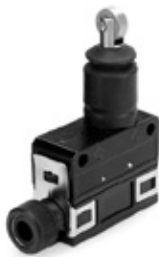
Series SL1: Cross Roller Plunger (90°; Rotated Plunger); 1 NC 1 NO SPDT Snap Action; Compression Fitting
