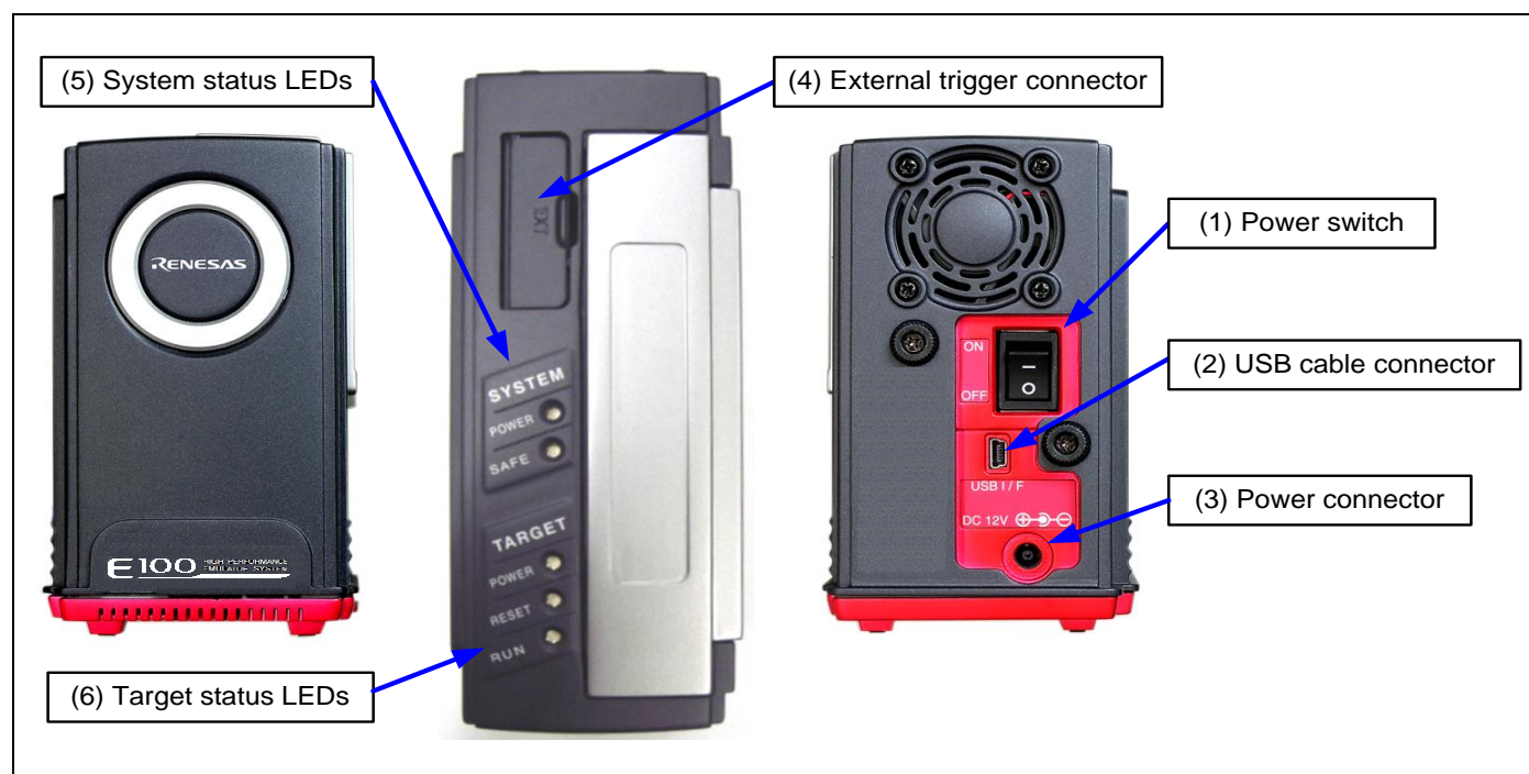
Figure 1.2 Names of the emulator parts
