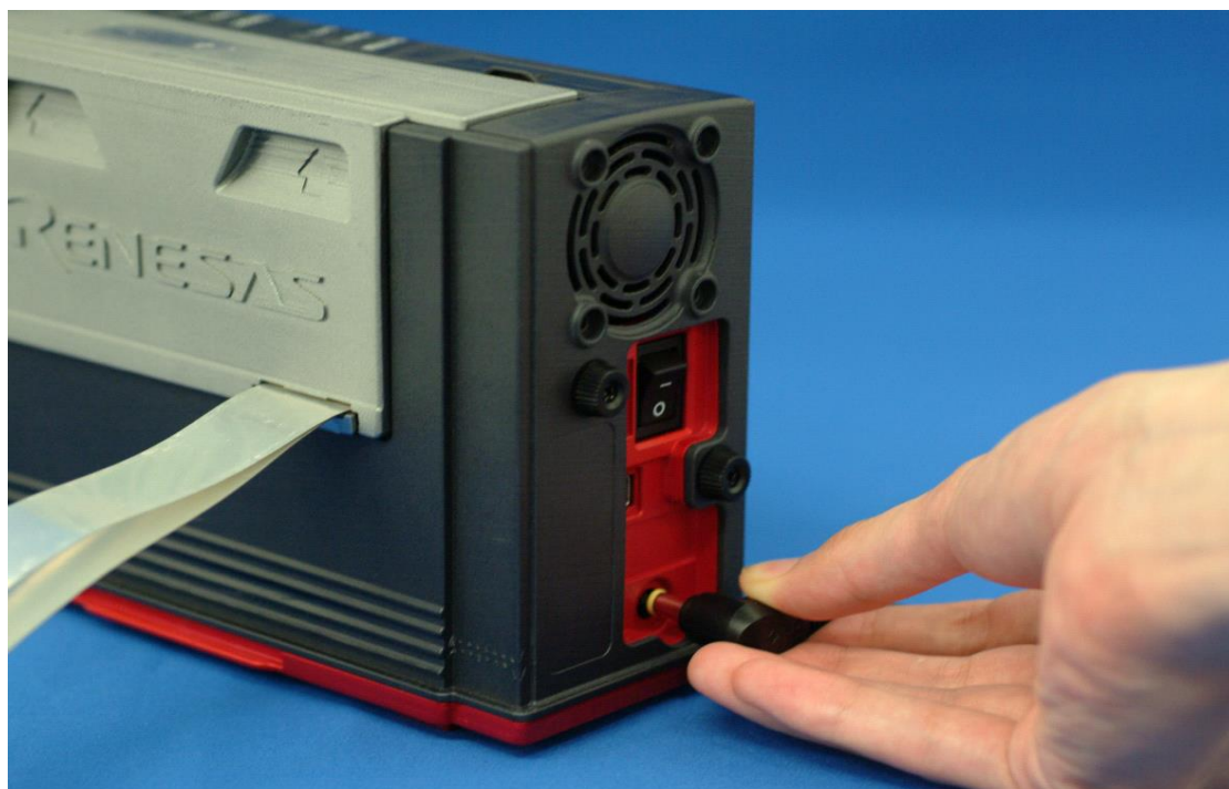
Figure 2.5 Connecting the emulator power supply
