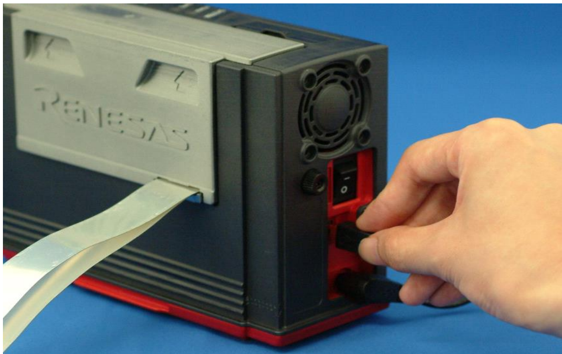
Figure 2.4 Connecting the host machine
