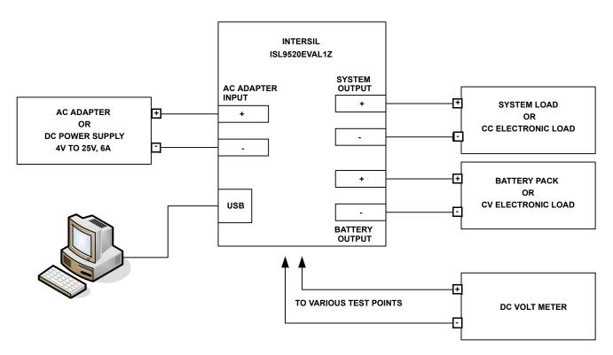
FIGURE 1. ISL9520EVAL1Z HARDWARE CONNECTION DIAGRAM
