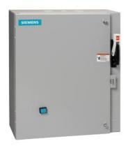
2-speed 3-phase motor starter Size 0 Two separate windings Constant horsepower Solid-state overload relays Low SPD OLR range 3-12A High SPD OLR range 3-12A 110V 50HZ / 120V 60HZ coil Combination type 30Amp disconnect switch Enclosure NEMA type 1 Indoor general purpose use
