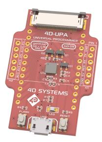
This connects to the pixxiLCD display through a 15-way-to-30-way cable.
