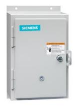
Non-reversing motor starter, Size 1, Three phase full voltage, Solid-state overload relay, OLRelay amp range 10-40a, 380 440/440 480V 50/60HZ coil, Non-combination type, Enclosure type 12, Dust/drip proof for indoors, Extra-wide enclosure
