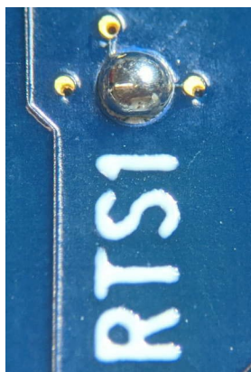
Figure 39. Single Soldering Iron on Solder Bridge
