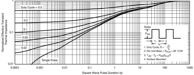
Normalized Thermal Transient Impedance, Junction-to-Ambient
