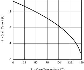
T<sub>C</sub> - Case Temperature (°C) **Current Derating\***
