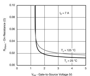
On-Resistance vs. Gate-to-Source Voltage
