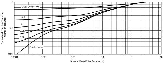
Normalized Thermal Transient Impedance, Junction-to-Foot
