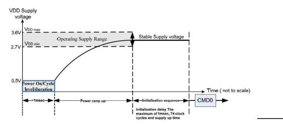
Host needs to keep power line level less than 0.5V and more than 1ms before power ramp up.
