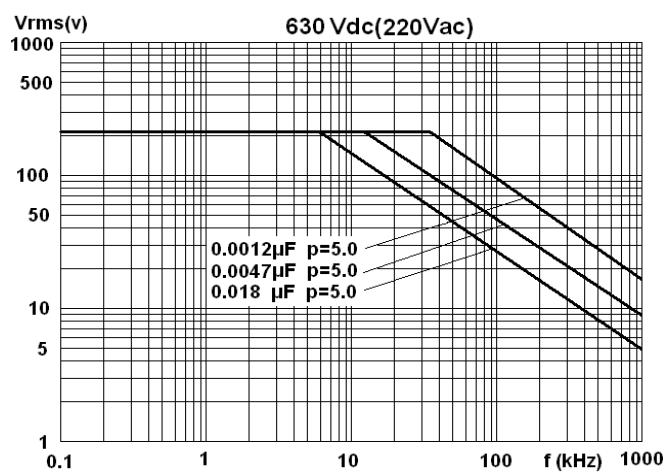
Note: sinusoidal wave-form, environment temperature  $\leq 85^\circ\text{C}$ , internal temperature rise  $\Delta T=15^\circ\text{C}$ , p (pitch) in mm..
