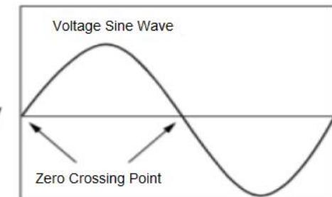
\*Zero crossing refers to the position where the sine wave voltage passes through 0V. See the figure on the right.
