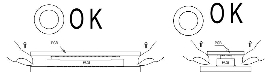
(2) When un-mating the connector, pull it out in parallel.
