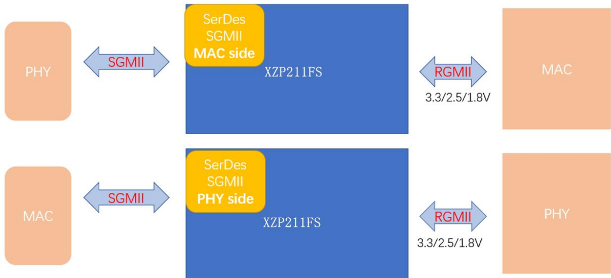
Figure 6. SGMII to RGMII Application
