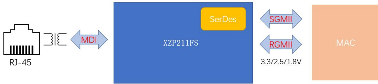
Figure 3. UTP (UTP<->RGMI / UTP<->SGMI) Application
