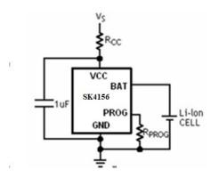
The small resistor  $R_{CC}$  will then be able to help the power dissipation when the charging current is large such as 1A in CC mode, and negligible when the charging current is small, such as 20mA in the final stage of CV operation.
