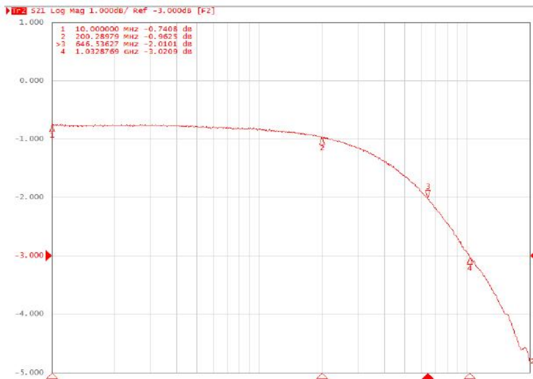
Fig 7. Switch Bandwidth or Insertion Loss
