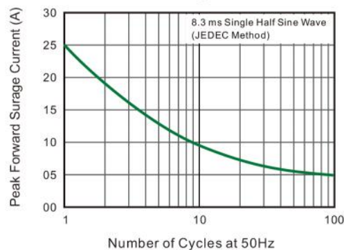
Fig.5 Maximum Non-Repetitive Peak Forward Surge Current
