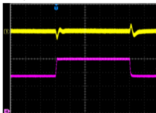
Load Transient@25% to 50% Load, 2.5A/µs
