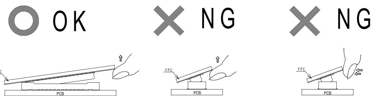
(3) IF THE FPC IS NOT RIGID, THE CONNECTOR CAN BE BROKEN. PLEASE CHECK THE ACTION OF THE FPC TO BE USED REPEATEDLY AT THE TIME OF TRIAL PRODUCTION. BE CAREFUL TO UN-MATE THEM FROM THE PITCH DIRECTION, PULLING IT FROM THE CORNER CAN ALSO RISK TO PUTTING STRESS ON CONTACTS.
