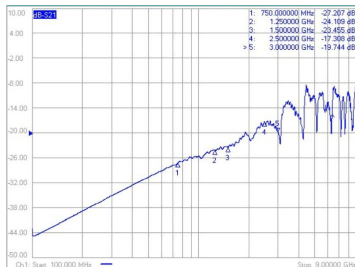
Fig.6 Switch Off Isolation
