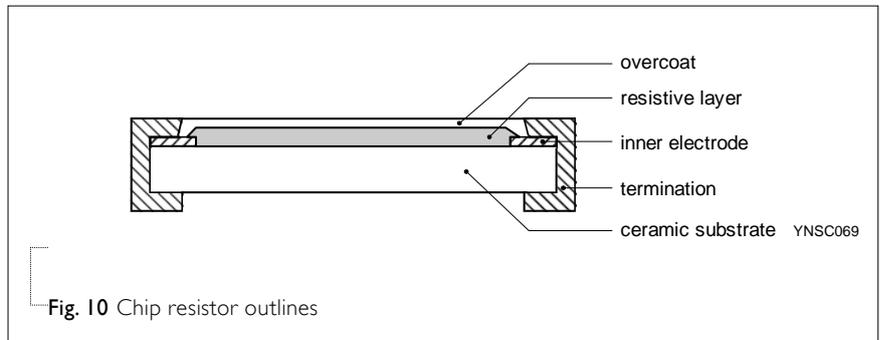
Fig. 10 Chip resistor outlines
