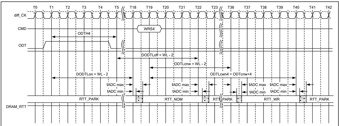
Figure 164 – Synchronous ODT example with BL=4, CWL=9, AL=10, PL=0; DODTLon/off=WL-2=17, ODTcwn=WL-2=17
