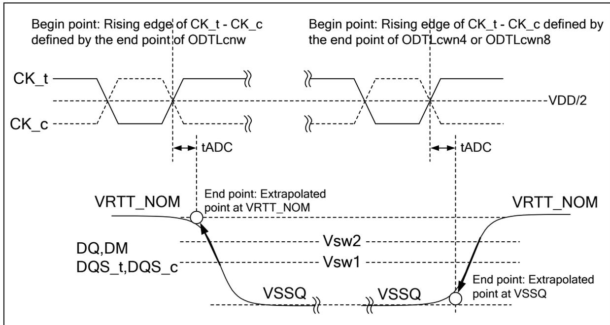
Figure 174 – Definition of tADC at Dynamic ODT Control
