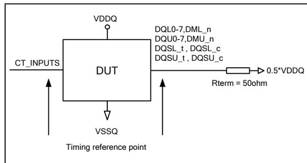
**Figure 194 – Connectivity Test Mode Timing Reference Load**
