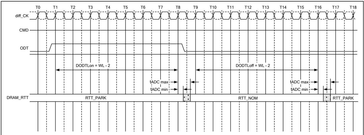
Figure 163 – Synchronous ODT Timing Example for CWL=9, AL=0, PL=0; DODTLon=WL-2=7; DODTLoft=WL-2=7
