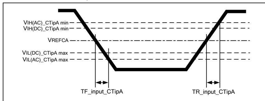
**Figure 156 – CS\_n and Input A Slew Rate Definition**
