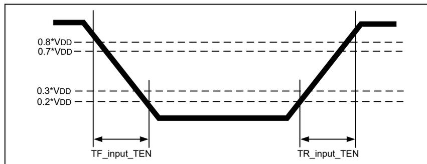
**Figure 155 – TEN Input Slew Rate Definition**
