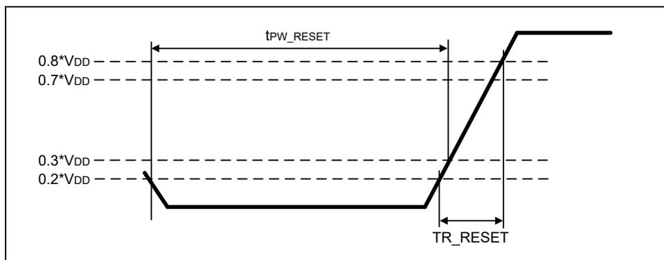
Figure 185 – RESET\_n Input Slew Rate Definition
