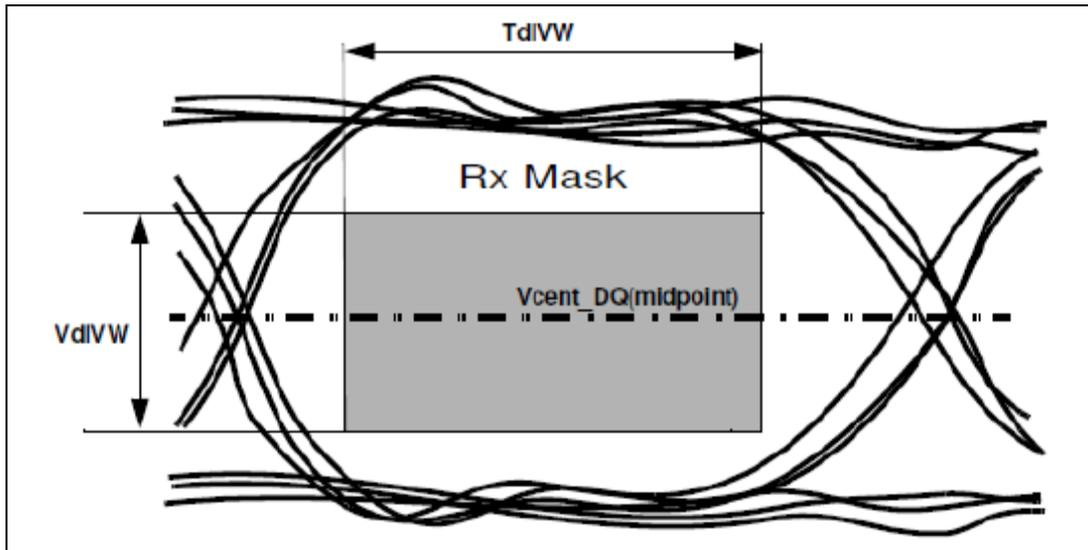
Figure 198 – DQ Receiver (Rx) compliance mask
