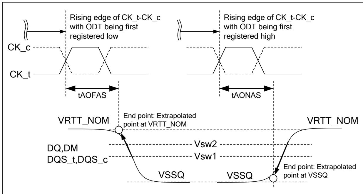
Figure 175 – Definition of  $t_{AOFAS}$  and  $t_{AONAS}$
