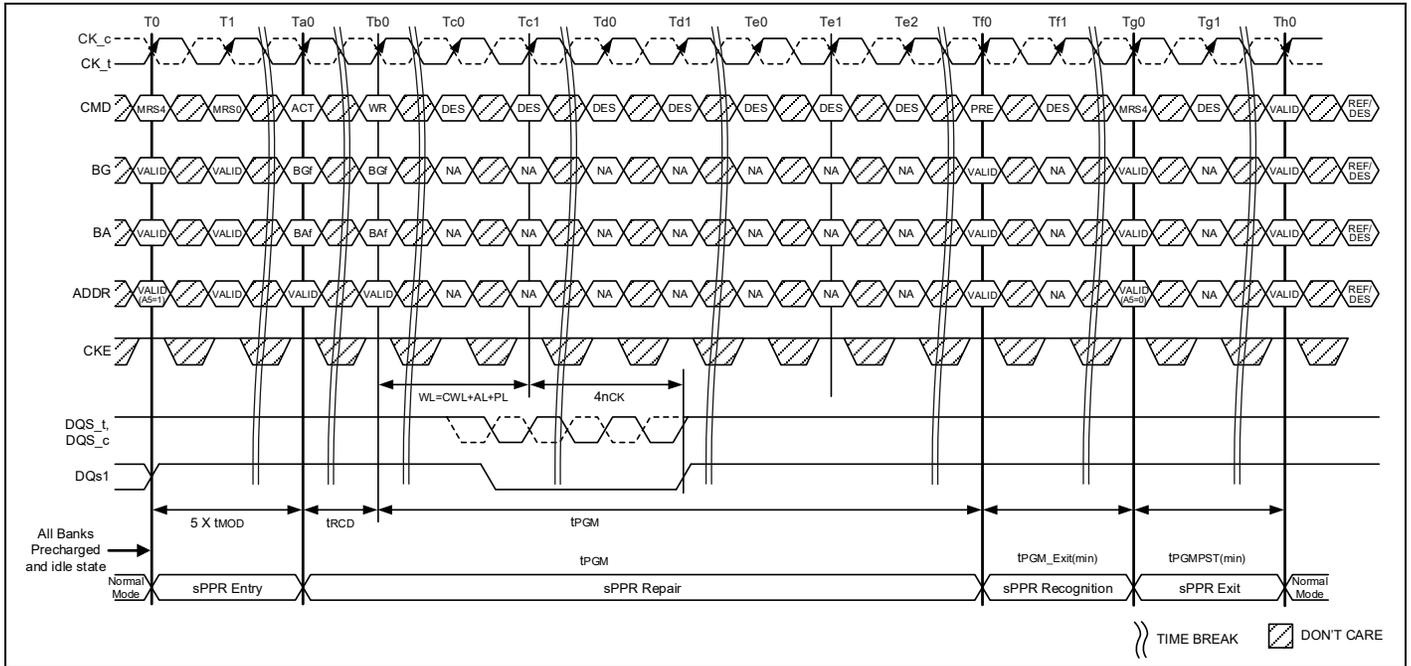
Figure 160 – Fail Row Soft PPR (WR Case)
