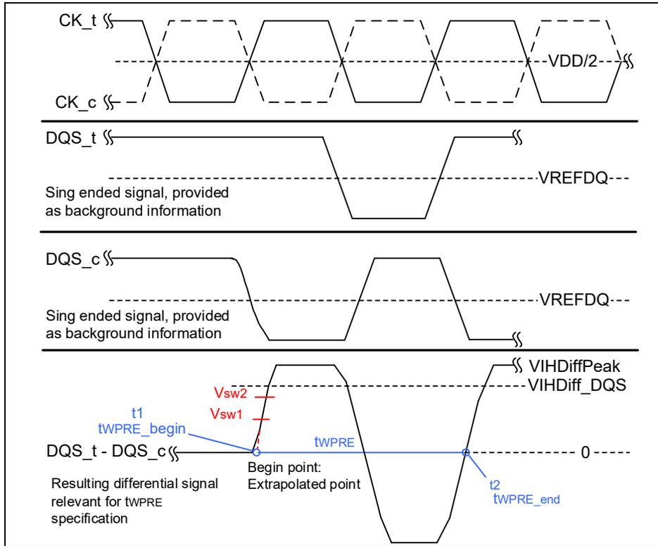
Figure 107 – Method for calculating tWPRE transitions and endpoints
