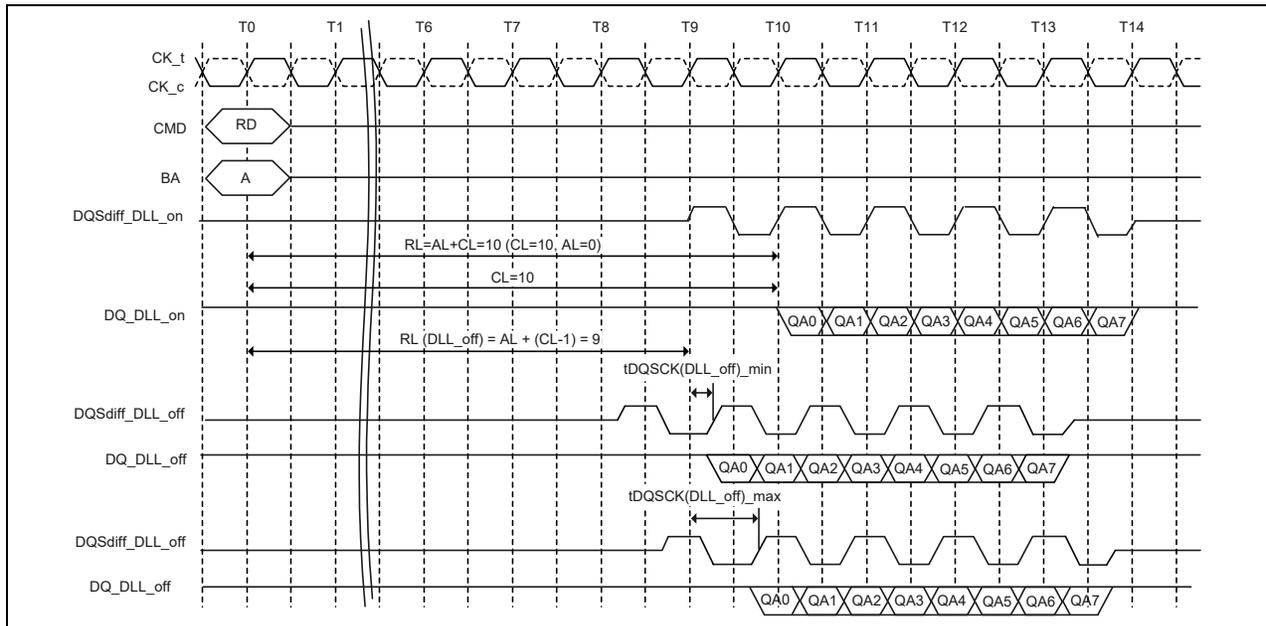
Figure 8 – READ operation at DLL-off mode
