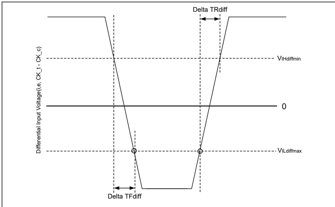
**Figure 182 – Differential Input Slew Rate Definition for CK<sub>t</sub>, CK<sub>c</sub>**
