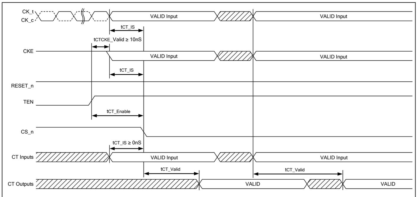
Figure 154 – Timing Diagram for Connectivity Test (CT) Mode
