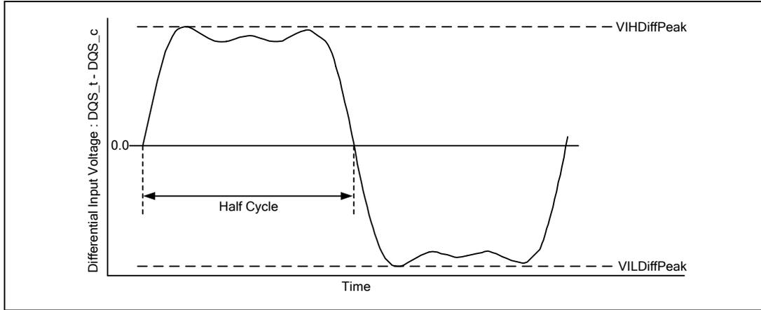
Figure 186 – Definition of differential DQS Signal AC-swing Level
