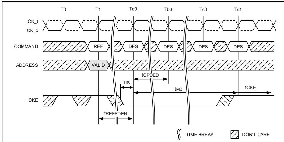
Figure 148 – Refresh Command to Power-Down Entry
