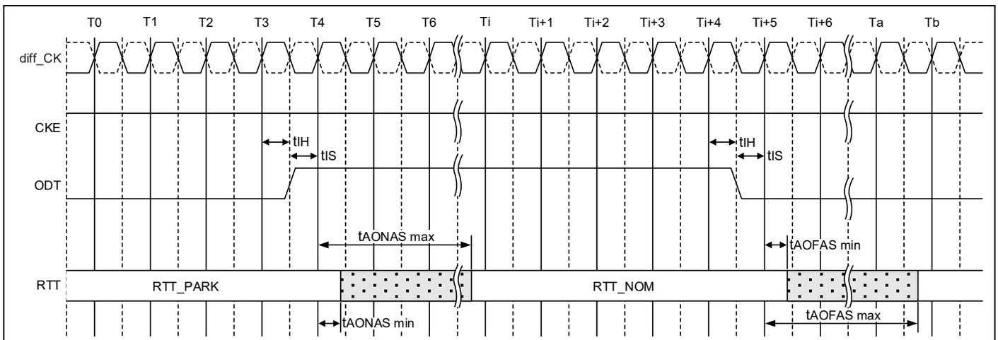
**Figure 169 – Asynchronous ODT Timing on DDR4 SDRAM with DLL-off**
