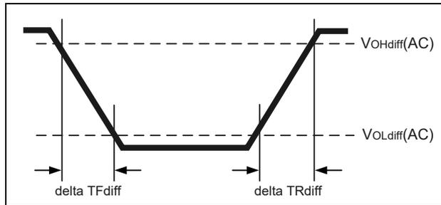
**Figure 192 – Differential Output Slew Rate Definition**
