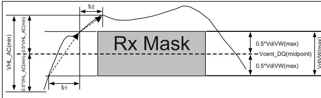
Figure 201 – Slew Rate Conditions for Rising Transition
