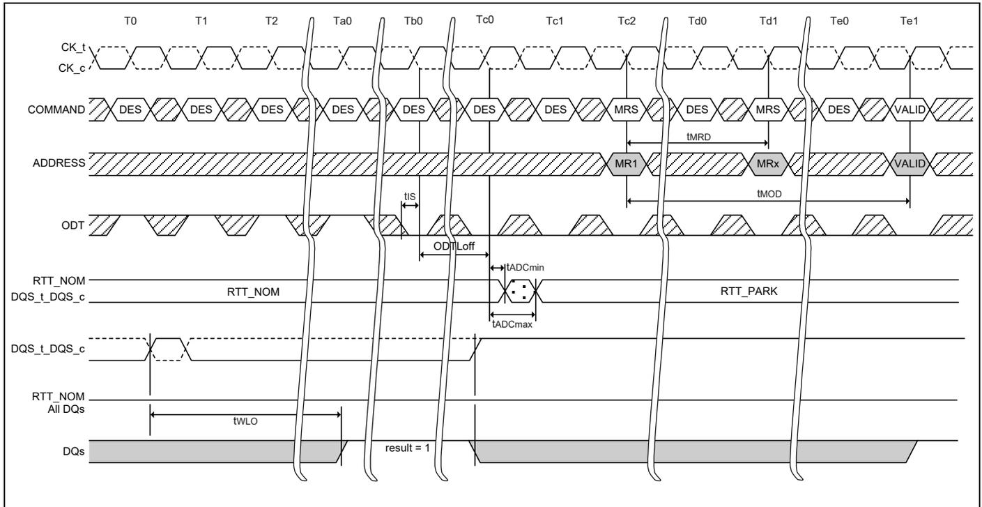
Figure 11 – Timing details of Write leveling exit
