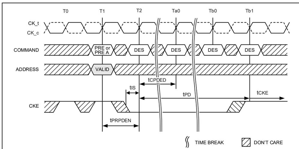
Figure 150 – Precharge/Precharge all Command to Power-Down Entry
