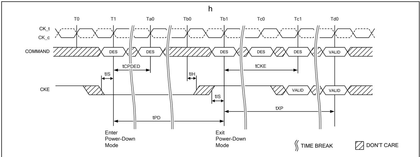
**Figure 147 – Precharge Power-Down Entry and Exit**
