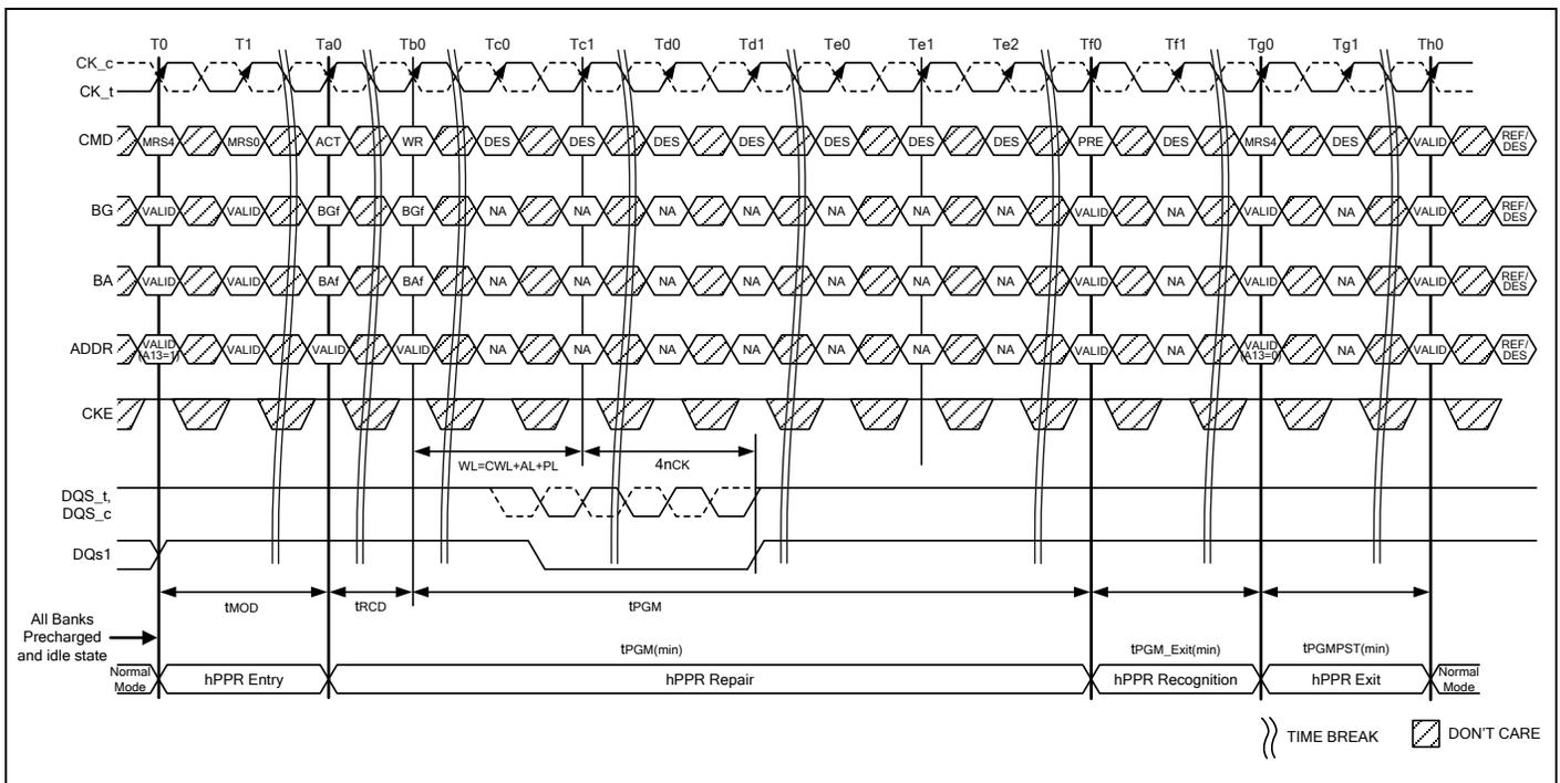
**Figure 159 – Hard Fail Row Repair (WR Case)**
