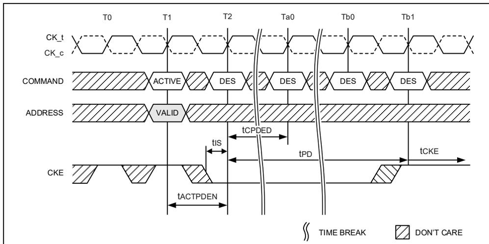
Figure 149 – Activate Command to Power-Down Entry
