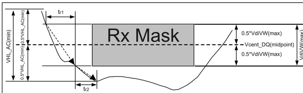
Figure 202 – Slew Rate Conditions for Falling Transition
