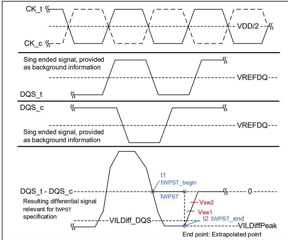
Figure 108 – Method for calculating tWPST transitions and endpoints
