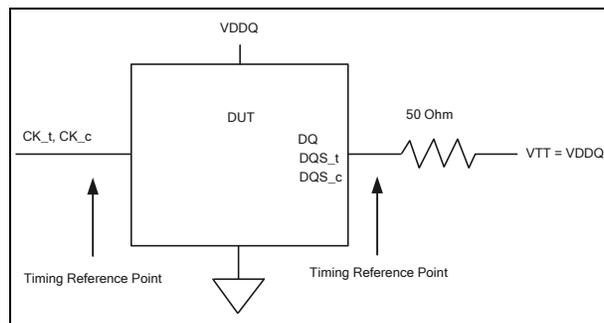
Figure 197 – Reference Load for AC Timing and Output Slew Rate
