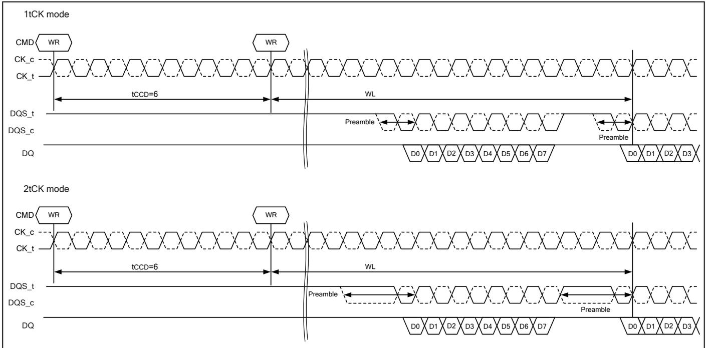
Figure 63 – 1tCK vs. 2tCK WRITE Preamble, tCCD=6 (AL=PL=0)
