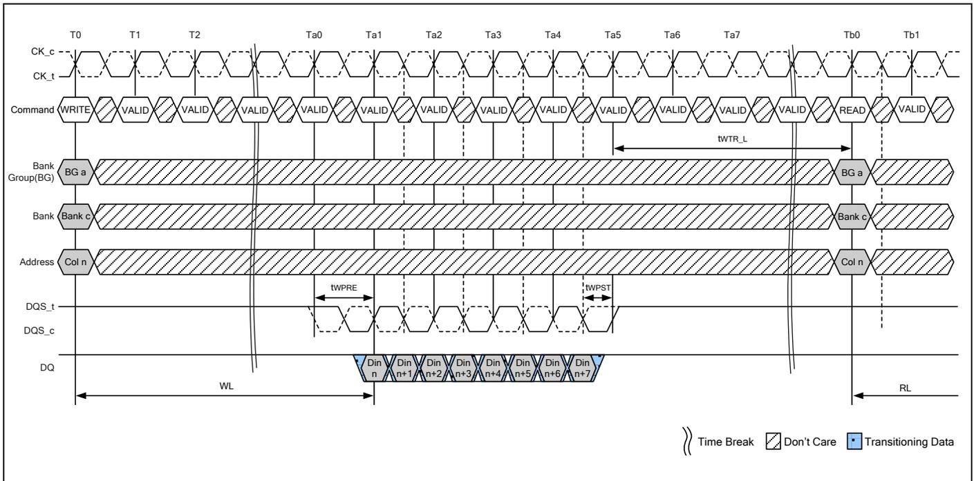
**Note:**  $tWTR\_L$ : Delay from start of internal write transaction to internal read command to the same Bank Group. When AL is nonzero, the external read command at  $Tb0$  can be pulled in by AL.
