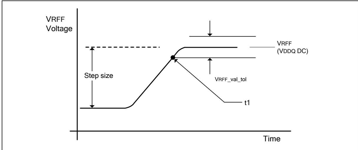
Figure 26 – VREF step single step size increment case
