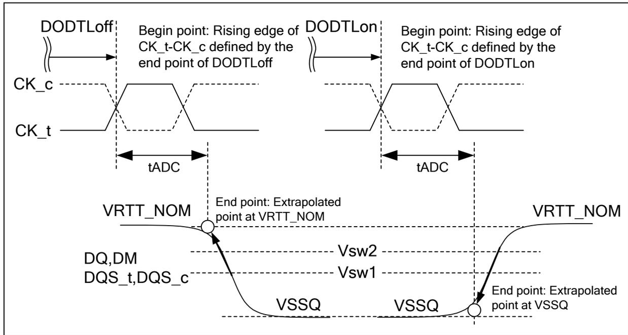
Figure 173 – Definition of tADC at Direct ODT Control
