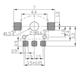
P.C.B thickness t=0.3~0.5 Tolerance:±0.1
