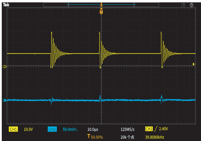
Figure 7, SW Switching & V_{out} Ripple Waveform ( I_{load}=0A )
