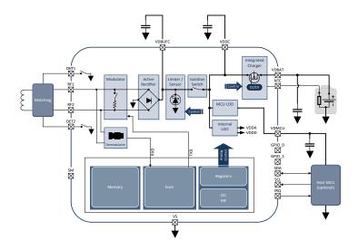
Renesas Electronics provides turnkey NFC wireless charging solution, combining PTX130W NFC wireless charging poller with PTX30W NFC wireless charging listener.
