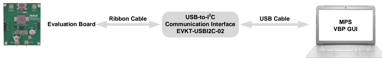
Figure 1: EVKT-MPQ4242B Evaluation Kit Set-Up
