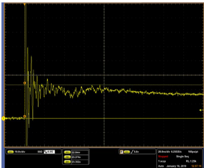
Figure 11: ISO10605 (C:330pF, R:330Ω) contact discharge plot at +8KV
