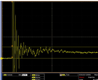
Figure 9: ISO10605 (C:330pF, R:330Ω) contact discharge plot at +8KV
