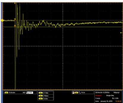
Figure 12: ISO10605 (C:330pF, R:330Ω) contact discharge plot at -8KV
