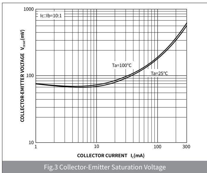
Fig.3 Collector-Emitter Saturation Voltage
