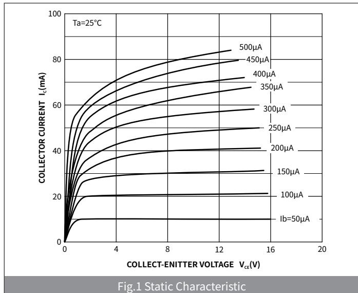
Fig.1 Static Characteristic
